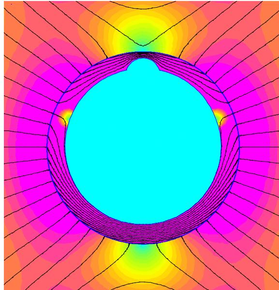
Comparing the flux density near the surface of the tubing near the wear and opposite the wear we see the effect with an amplitude of around 2.5 mT or about 25 gauss in this simulation. This is well within the capabilities of a standard linear Hall Effect sensor.
