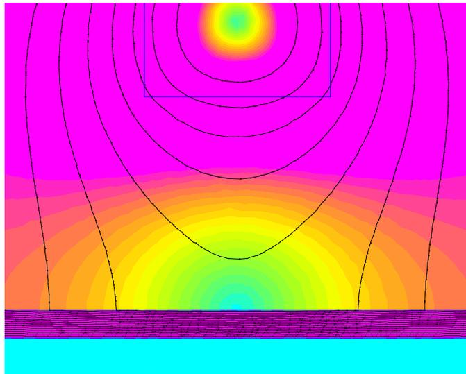
The second diagram shows the same area when a small divot of tubing material is removed from the inside surface of the tubing. Notice the increase in flux density just above the tubing along the vertical axis of the coil.
